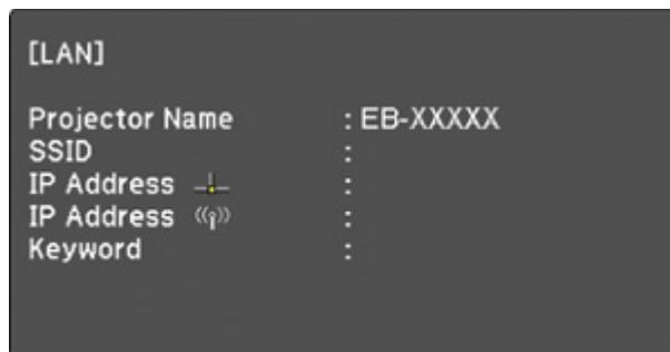
3. Verify that an SSID and IP address are displayed, then remove the wireless LAN module from the projector.
